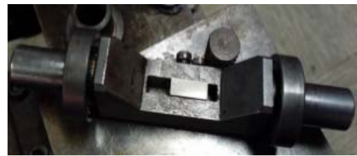
Fig. 3. Placing the block in the bracket
