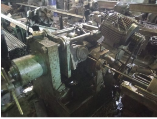
Fig. 2 Straightening Process of round bar in Two Cross-Roll straightening machine (SMH-25).
