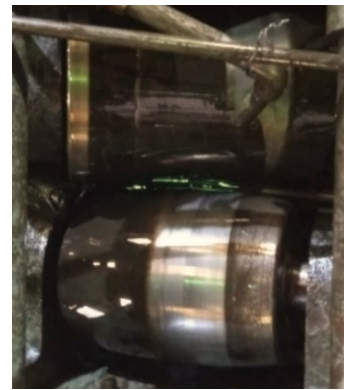
Fig. 1a Convex and Concave Rollers showing round bar in between during the straightening process.
