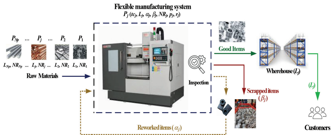
Figure 1. Flexible manufacturing system producing multi-products and prone to random failures, scrap, and rework
