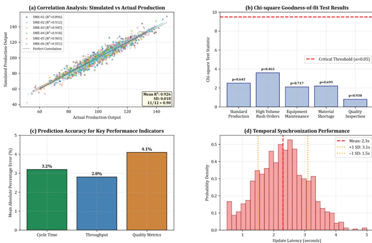
Figure 1. Comprehensive Digital Twin validation analysis across twelve SMMEs pilot implementations. (a) Correlation analysis between simulated and actual production outputs showing R^2 values and regression lines for each organization. (b) Chi-square goodness-of-fit test results across different production scenarios with acceptance thresholds. (c) Prediction accuracy analysis for key performance indicators including cycle time, throughput, and quality metrics. (d) Temporal synchronization performance showing latency distributions and real-time update frequencies.
