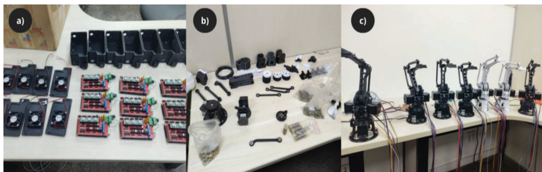
Figure 3. Evidence of the Robot Manufacturing Stage (a) Raspberry Assembly (b) Robot Parts (c) Assembled Robots (Source: Authors own work)
