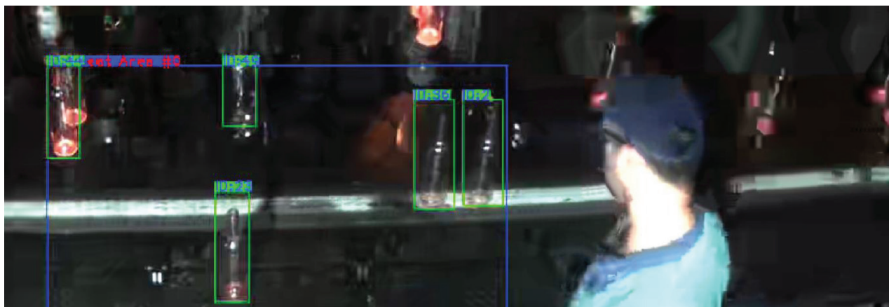
Figure 13. With a QP offset of 11 and BR=300 kbps, there is a quality difference between ROI and remaining image
