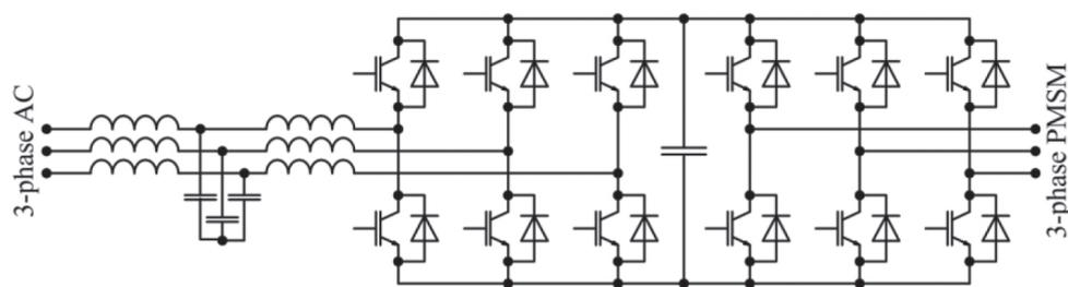
Figure 5. Simplified circuit diagram of ACS800
