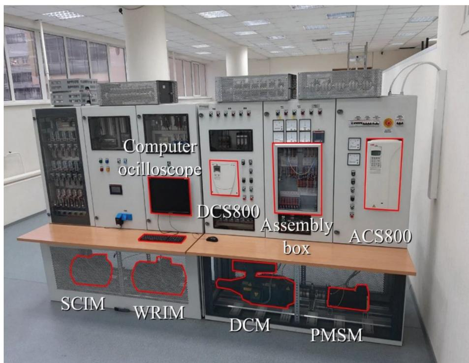
**Figure 1.** Photo of the test bench. The side with DCM and PMSM is shown. From left to right cabinets with: relays, PLC and touchscreen, sensors and computer oscilloscope, DCM with DCS800, indicators and assembly box, PMSM and ASC800.
