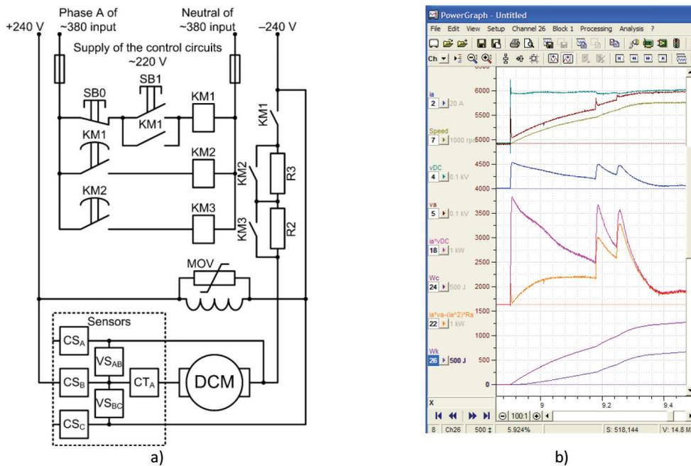
**Figure 8.** Direct on line starting of the DCM a – Electrical circuit: CSA, CSB, CSC are the current sensors, VSAB and VSBC are the voltage sensors and CTA is the current transformer. b – transients observed.
