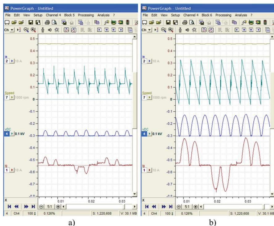
Figure 11. Operation of the DCM fed from controlled rectifier. From top to bottom: speed, armature voltage, armature current, grid current: a—idle mode at 1000 rpm; b—10 A load at 1000 rpm.
