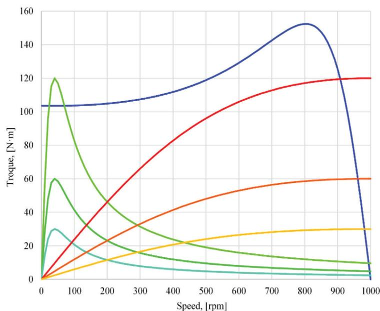
**Figure 3.** WRIM is loading SCIM in braking mode: blue—rated speed-torque curve of the SCIM under test; red to orange—mirrored speed-torque curves of WRIM with additional resistors in the rotor windings with different excitation currents flowing in the stator winding; lime to cyan—mirrored speed-torque curves of WRIM without additional resistors in the rotor windings with different excitation currents flowing in the stator winding.
