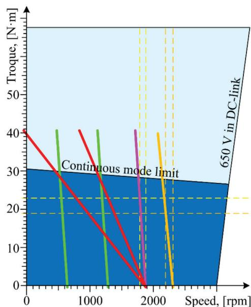
**Figure 2.** Operating region of PMSM (generator mode) and a set of speed-torque curves of DCM (driving mode): dark blue—area of continuous operation of the PMSM; light blue—area of short-term operation mode of the PMSM; magenta—rated speed-torque curve of the DCM; orange—speed-torque curve in the field weakening mode; red—set of speed-torque curves with additional resistance in the armature winding; lime—set of speed-torque curves for various armature voltages.
