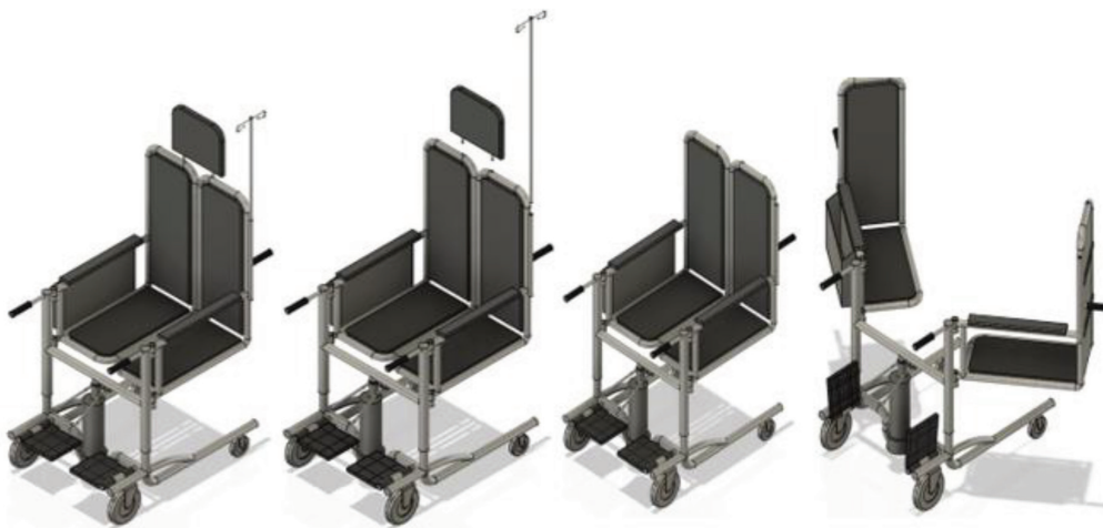
Figure 6. Design of the Transfer Wheelchair Prototype
