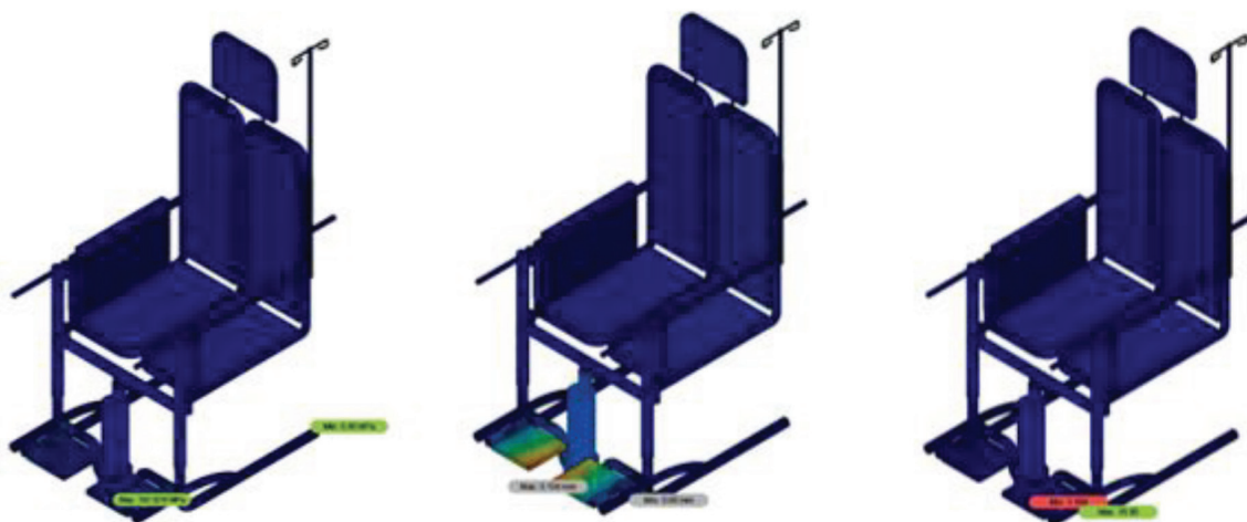
Figure 7. Stress, Deformation, and Safety Factors for Transfer Wheelchairs
