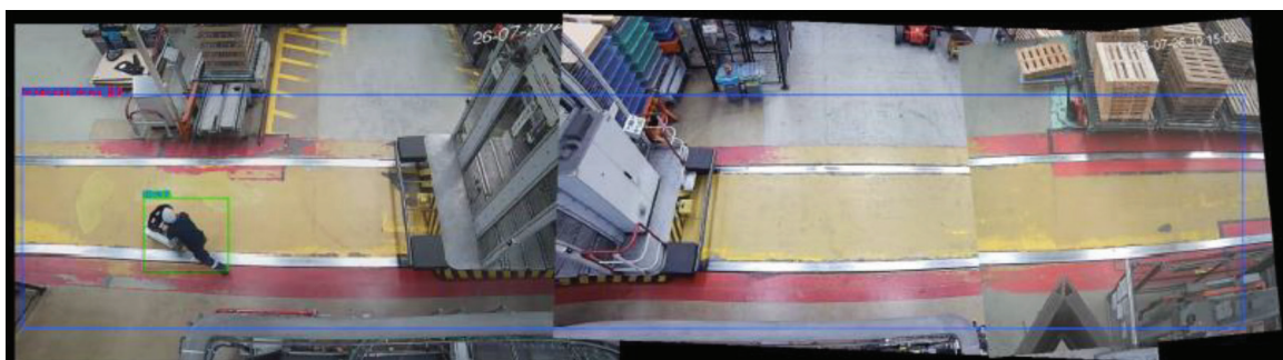
Figure 9. Detection of people within the ROI defined by the user, covering the combined 3 camera FOVs
