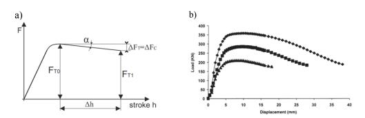
Figure 11 – Theoretical (a) and experimental (b) Load - stroke diagram of forward extrusion [34]
