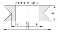
Figure 4 - New proposed shape for ring – test [7]
