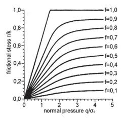
Figure 1 – Friction stress in general friction model [7]
