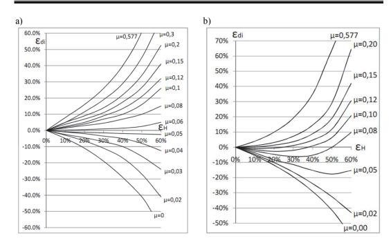
Figure 3 - Friction calibration curves obtained by Male and Cockroft (a) and Avitzur (b) [14],[15]
