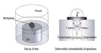
Figure 12 – T-shape compression test [35]
