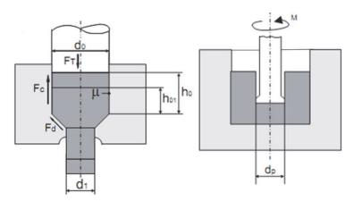
Figure 10 - Forward bar extrusion [31] and twist extrusion [33]:
