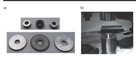
Figure 8 – Ring test samples (a) and ring compression process (b) [5]
