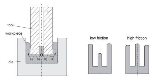
Figure 13 - Left: Double backward extrusion ("a" and "b" are directions of material flow),
