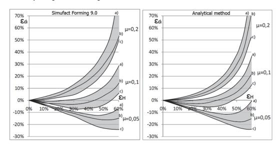
Figure 7- FCC for different ring thicknesses (a - 30:15:8 mm, b - 30:15:10 mm, c - 30:15:12 mm) in FEM simulation (left) and analytical calculations (right) [24]
