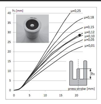
Figure 14 – Friction calibration curves obtained by Simufact Forming 9.0 [27]
