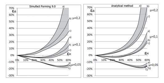
Figure 6 – FCC for different inner ring diameters (a – 30:12:10 mm, b – 30:15:10 mm, c – 30:18:10 mm) in FEM simulation (left) and analytical calculations (right) [24]
