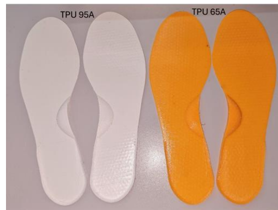
Fig. 10 3D-printed insoles made of TPU with hardness levels of 95A and 65A
