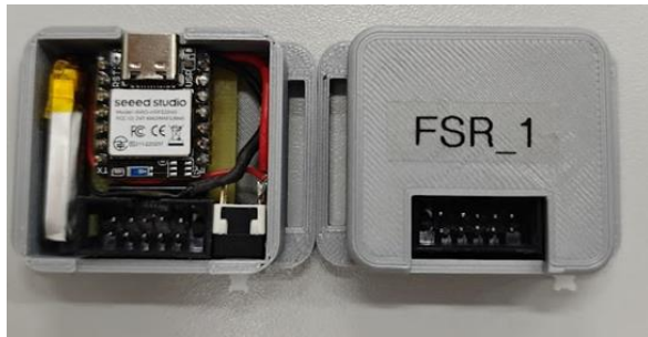
Fig. 7 Smart insole electronics housed in a plastic enclosure
