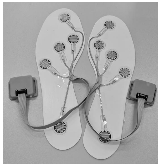
Fig. 1. Smart insole system: (a) overview of the integrated components, (b) developed hardware prototype
