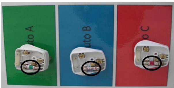
Figure 6. Areas with colour codes for each type of fuse (from left to right, 2, 7 and 13 amperes)
