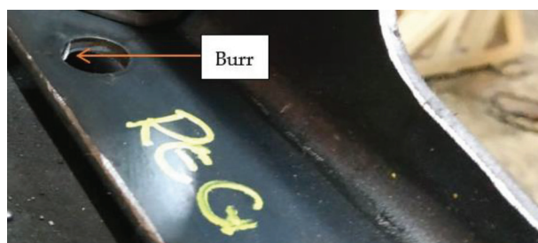
Figure 5. Detail of Burr on a Press Part
